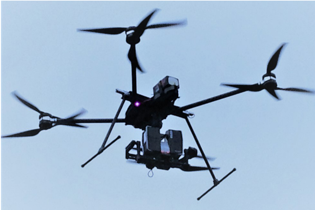
Think 3D's STORMBEE in action: The innovative scanning solution that combines the FARO Laser Scanner Focus 3D X130 with a drone.
