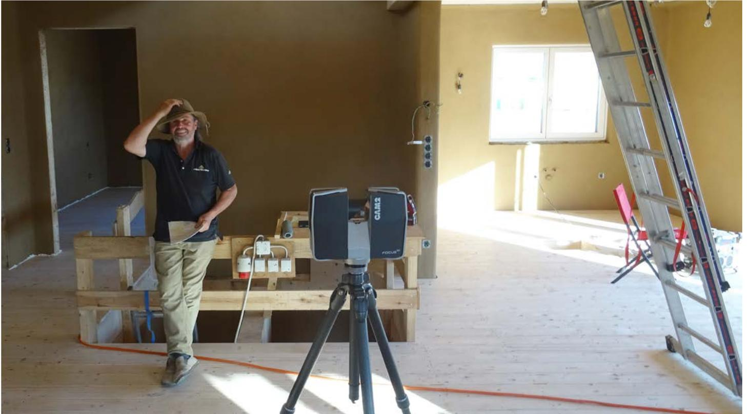
*With the FARO Focus<sup>3D</sup>, the dimensions required to construct the staircase are recorded quickly and efficiently.*
