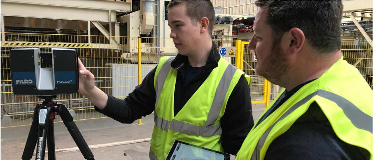
Kronospan use the FARO Focus Laser Scanner to survey their site.
